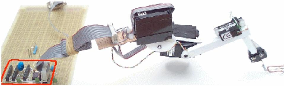
**Figure 5:** An experimental robot leg made from model aeroplane servos. The knee joint weighs only 6g. The microcontroller and three H bridges outlined in red on the left are all the electronics needed to control the leg.
