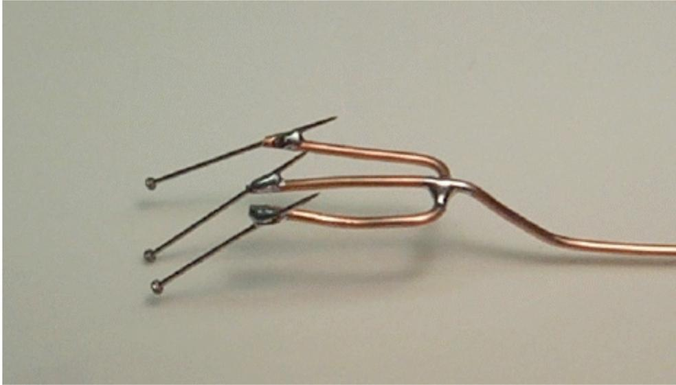
**Figure 4:** A crude claw made from sewing pins soldered to copper wire. This supported a load of over 1.5kg. Dragging it over the foam with no extra downward force was sufficient to lock it into the surface. It could be removed by reversing its direction; this required no discernible force at all.
