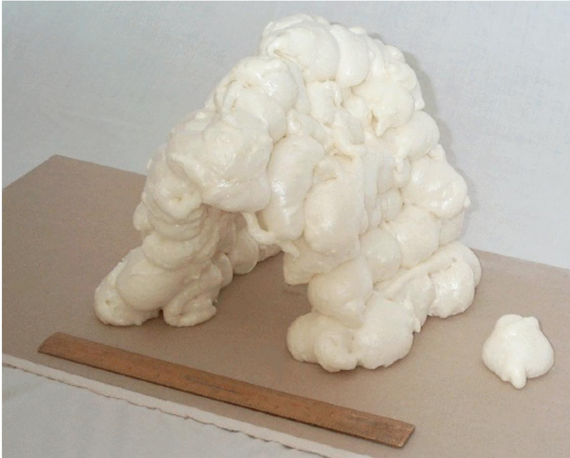
**Figure 1:** A small arch made by repeatedly depositing by hand lumps of diphenylmethane 4,4'-diisocyanate foam similar to the example on the right. In front is a foot rule.
