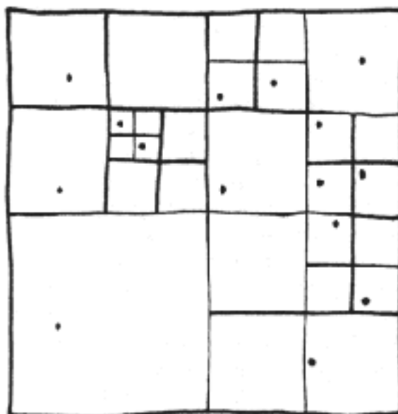
6(i)—A quad-tree divided down until each square contains at most one data point.
