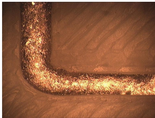
Figure 4: Results from the syringe with a heating jacket. The track is 1.2 mm wide.
