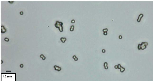
Fig. 1. Image of beads following suspension and settling in excess buffer showing beads aggregating and annealing.
