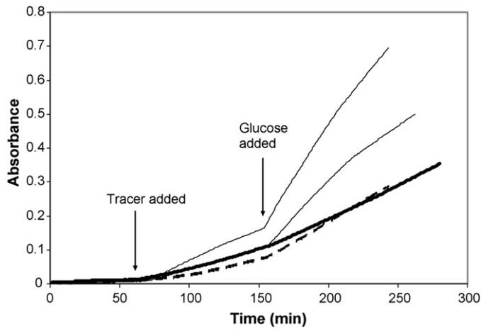
**Fig. 5.** Effect of D-glucose addition to the diffusion time course of tracer through a ConA dextran pore filled membrane (bold solid line 10 mM, bold broken line 20 mM, solid line 30 mM, broken line 40 mM).
