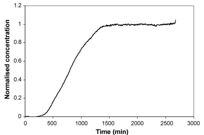
Fig. 4. Time taken for tracer concentration to reach equilibrium across a pore-filled membrane (recirculation flow 1.02 g/min).
