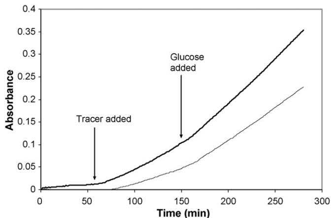
**Fig. 7.** Comparison of glucose effect between first (solid line) and last (broken line) experiments in the sequence.
