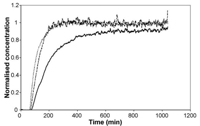
Fig. 3. Effect of recirculation flow rate on time taken for tracer concentrations to reach equilibrium across an unmodified membrane (short dash 1.24 g/min, long dash 1.02 g/min, solid 0.83 g/min).
