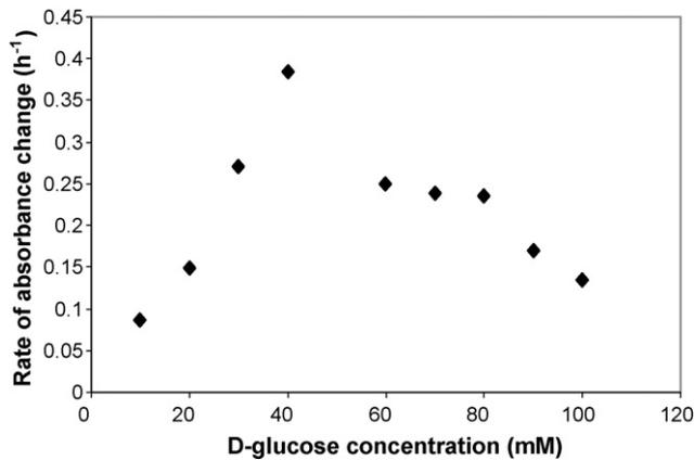
**Fig. 6.** Effect of D-glucose concentration on the diffusion rate of tracer through a ConA dextran pore-filled membrane.
