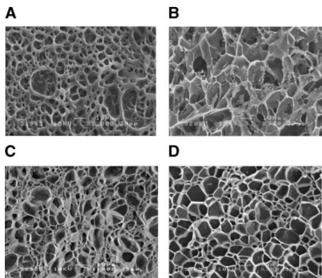
**Figure 5.** SEM showing the three-dimensional structure of the antigen-responsive hydrogel in (A) pH 7.4 buffer and (B) pH 7.4 buffer containing 0.1 mg/mL sodium fluorescein; and a control gel (containing BSA in place of the antibody) in (C) pH 7.4 buffer and (D) pH 7.4 buffer containing 0.1 mg/mL sodium fluorescein.
