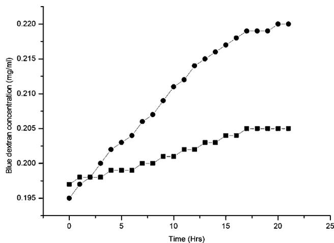
**Figure 7.** Diffusion of Blue dextran (6,000 kDa, 0.2 mg/mL) into a hydrogel slab in the presence (▲) and absence (■) of 0.1 mg/mL sodium fluorescein at pH 5.0.
