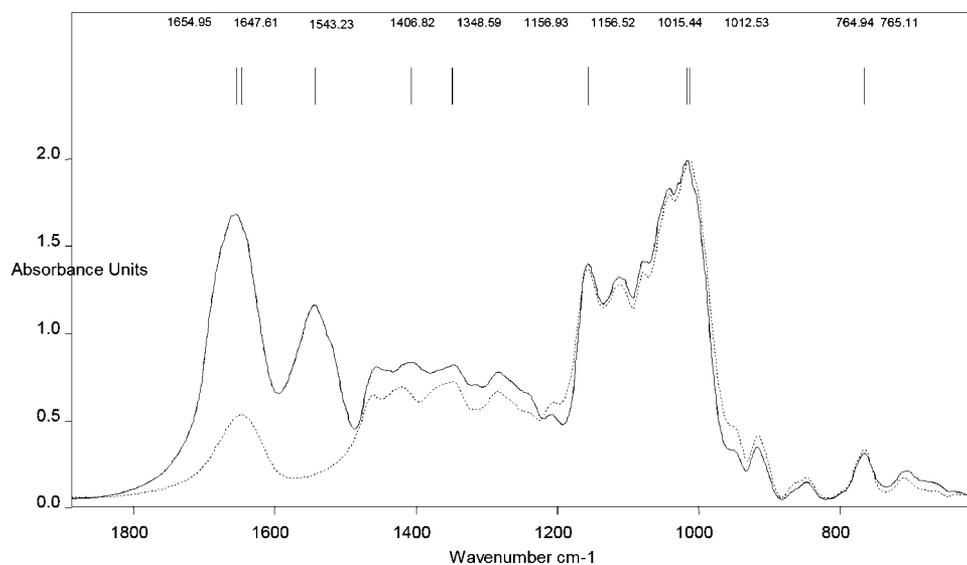
**Figure 3.** FTIR spectra of the FITC-Dextran-DVS-antibody hydrogel.
