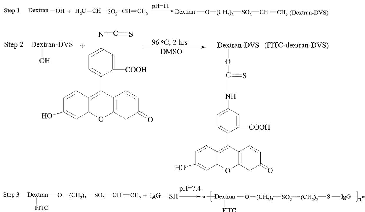
**Figure 1.** The chemistry of the FITC-dextran-DVS-antibody hydrogel preparation.
